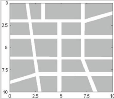
**[Network]** This example of a network  $K \subset \mathbb{R}^2$  is a set of roads of a 2-dimensional network (in white). The first question studied in this book is to construct a *celerity regulator* indicating at each instant and at each position the velocity advised to any vehicle to remain on the road. We add other specifications (travel duration, acceleration, congestion, collision avoidance, etc.).
