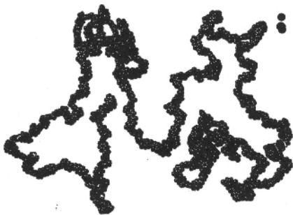
Figure 1.5 Representation of the Gaussian coil conformation of a chain molecule, the monomer units being represented by dark spheres, for details see text.
