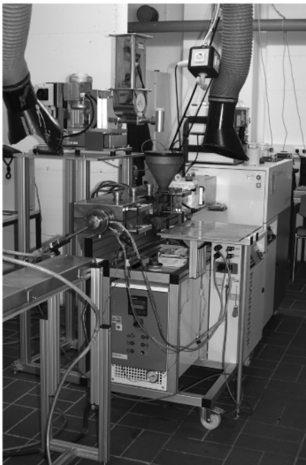
Figure 1.7 Lab-type extruder with the extrusion die pointing to the reader.
