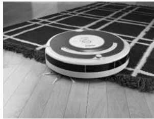
Fig. 1.39. The vacuum robot Roomba, employing a differential-drive kinematics, autonomously sweeps and cleans floors (courtesy of I-Robot Corp)
