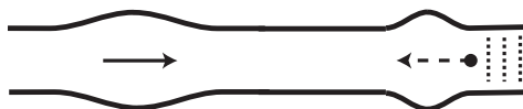
Fig. 2.7.3. A wave moving in one direction along an elastic tube may be reflected totally or partially by an obstacle, resulting in a secondary wave moving in the opposite direction.
