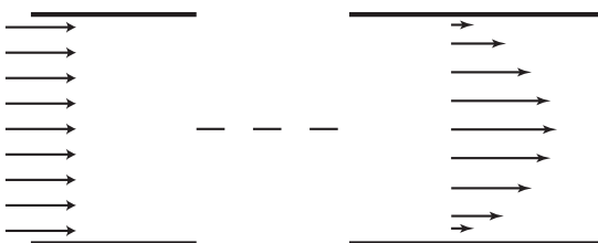
Fig. 2.5.2. Flow in the entrance region of a tube provides another example of acceleration and deceleration in space . If fluid enters with uniform velocity, elements of the fluid along the tube axis must accelerate to meet the maximum velocity in Poiseuille flow, while fluid elements near the tube wall are slowed down by the viscous resistance and condition of no-slip at the tube wall.
